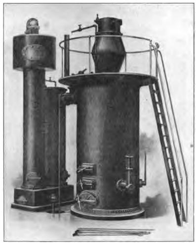
Fig. 59. — Crossley Suction Gas-Producer.
