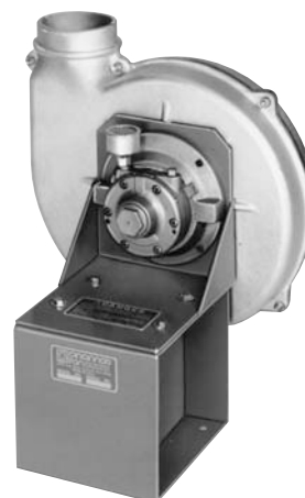
PB-9 with air motor. Cast aluminum blower with non-electric motor required to handle highly volatile substances at variable flow rates.
